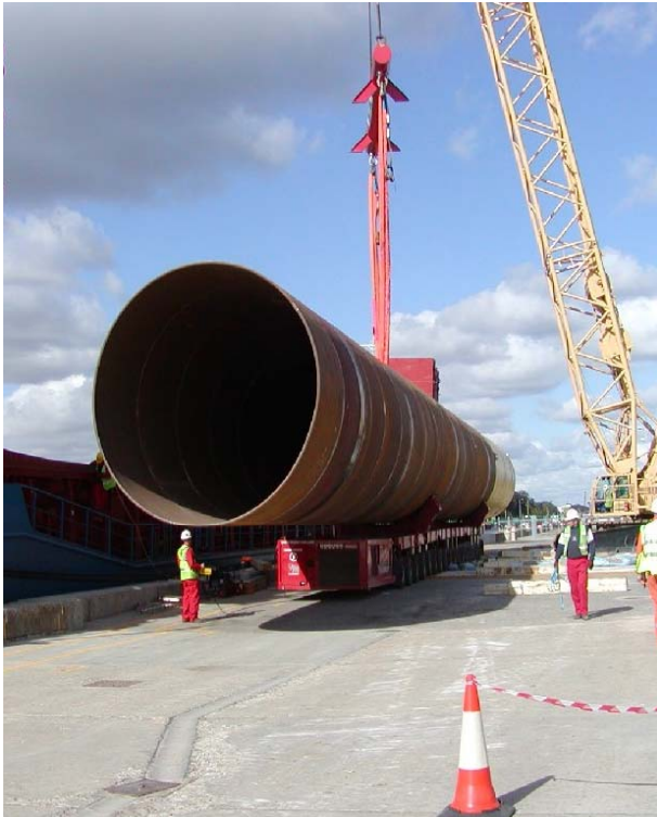
Monopile delivered to harbor
