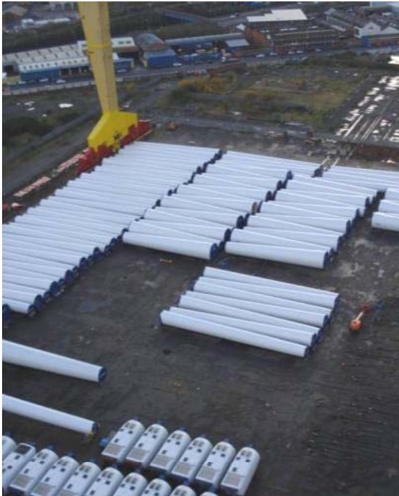
Port storage for towers & nacelles
