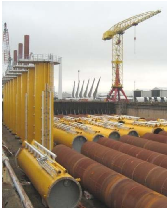
Port storage for monopiles
